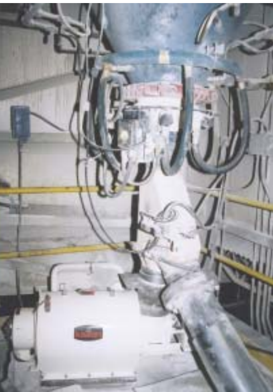
CENTRI-SIFTER centrifugal screener fits into tight space. Access door allows quick inspection, cleaning and screen changing. Slide gate valve (rear) controls flow rate of powder discharged from the blender into the screener.
