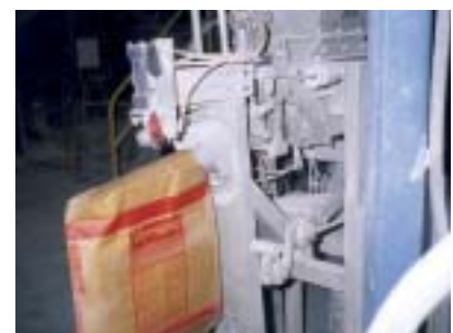
A 4000-lb (1814 kg) batch of polymer concrete is bagged in 15 minutes.
