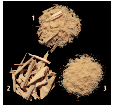
Wood: 1) mixture of undersize chips and powder, 2) on-size chips, and 3) low bulk density fines — as separated by screen vibration and airflow.
