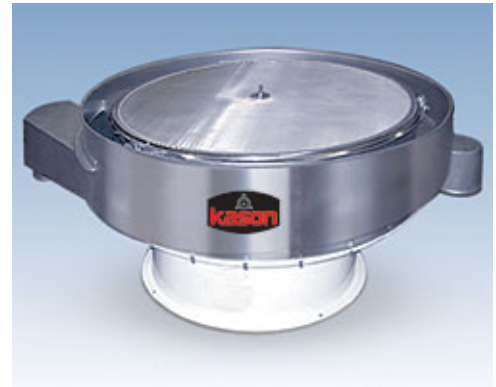
"External Cascade" deck of 60 in. (1524 mm) diameter Vibroscreen® separator (shown with lid removed) allows large percentages of oversize particles to cascade 360° around the screen periphery, eliminating a capacity restriction associated with conventional discharge spouts.
