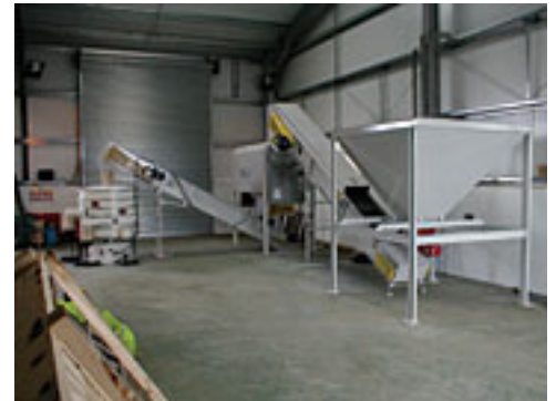
Incoming bottles drop through the hopper onto a belt that feeds the popper unit and sander (right rear), which break the glass into particles of 0.75-in. (19 mm) or less. The glass is then fed to the Kason classifier (left rear).
