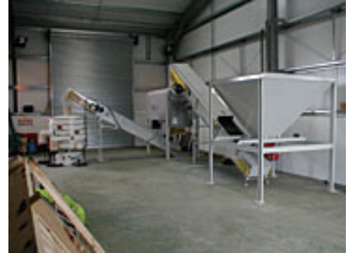
Incoming bottles drop through the hopper onto a belt that feeds the popper unit and sander (right rear), which break the glass into particles of 0.75-in. (19 mm) or less. The glass is then fed to the Kason classifier (left rear).
