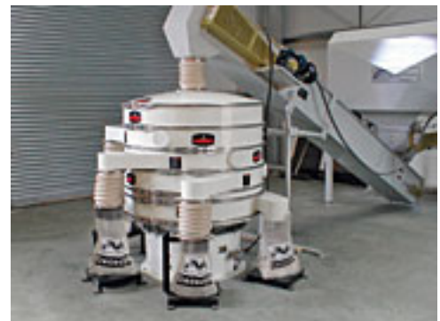
The Kason classifier is a vibratory separator that contains several screens to separate material by size. The unit is vibrated in an eccentric manner by a gyratory motor and is supported by rugged springs that allow free movement.
