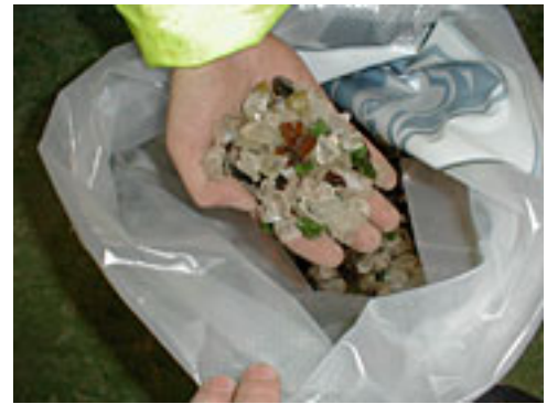
The glass products separated by the Kason classifier range from dust and fine material that can be used for shot-blasting to decorative glass for landscaping.
