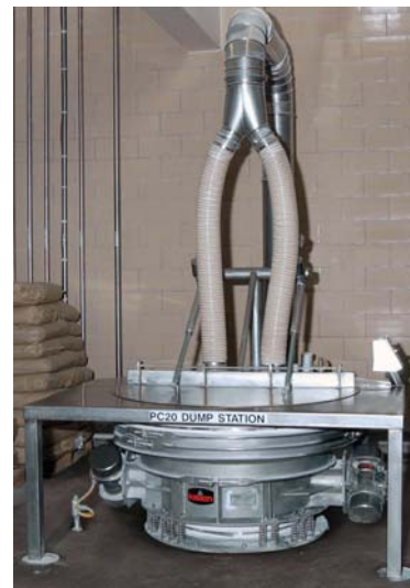
Waist-high table, 80 in. (2032 mm) wide and 68 in. (1727 mm) long, accommodates two operators simultaneously opening and emptying bags.
