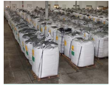
Delivered in bulk bags or truckloads, 100% recycled, granulated rubber is obtained from tire processors in sizes from 0.75 in. (19.05 mm) down to 10 mesh (2000 microns).
