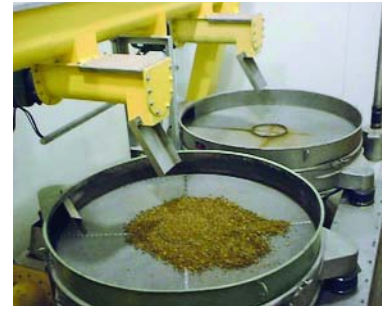
At 84-in. (2134-mm) in diameter, this Kason model K84-1-SS (foreground) is reportedly the largest circular screener made in Australia.
