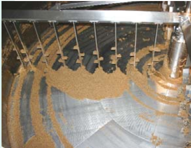
A view into top of a brew vat, showing the solids that must be washed away between brewings.
