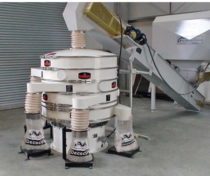
The Kason classifier is a vibratory separator that contains several screens to separate material by size. The unit is vibrated in an eccentric manner by a gyratory motor and is supported by rugged springs that allow free movement.
