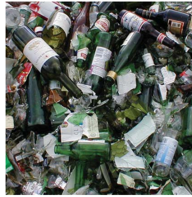
Glass bottles and jars of all kinds, with labels and metal foil attached, are the feed for the Lewis glass-recycling plant.
