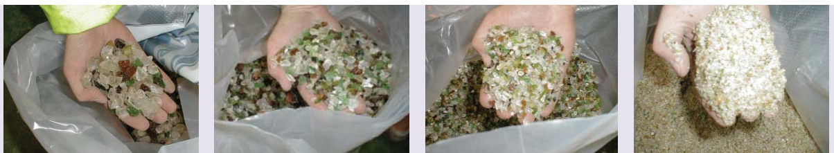
The glass products separated by the Kason classifier range from dust and fine material that can be used for shot-blasting to decorative glass for landscaping.
