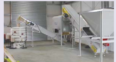
Incoming bottles drop through the hopper onto a belt that feeds the popper unit and sander (right rear), which break the glass into particles of .75 in. (19 mm) or less. The glass is then fed to the Kason classifier (left rear).
