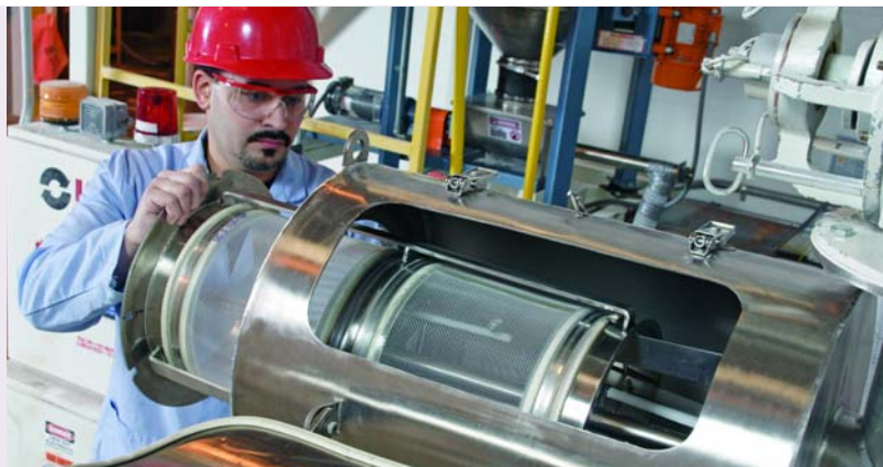
Cylindrical screen and helical paddles slide out of the Centri-Sifter MO screener end for thorough washdown and rapid screen changes.
