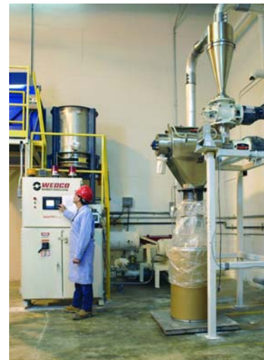
Wedco Polisher (left) is a continuous inline mixer that improves the flow properties of materials. After mixing and surface-smoothing, particles are transferred to Kason Corporation's Centri-Sifter MO screener (right) that separates on-size particles from oversize agglomerates.
