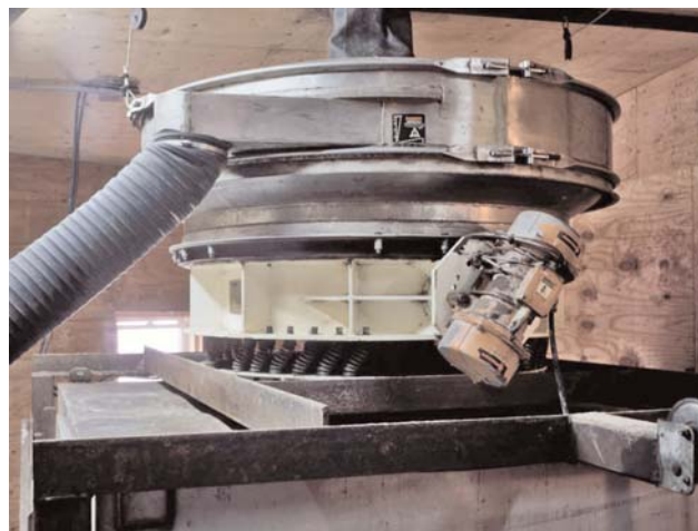
Low-profile 72" (1829mm) diameter Flo-Thru Vibroscreen® separator fits in 60" (1524mm) space between ceiling and holding bin that receives on-size material. Oversize particles >0.125" (3.175mm) exit through side discharge spout.
