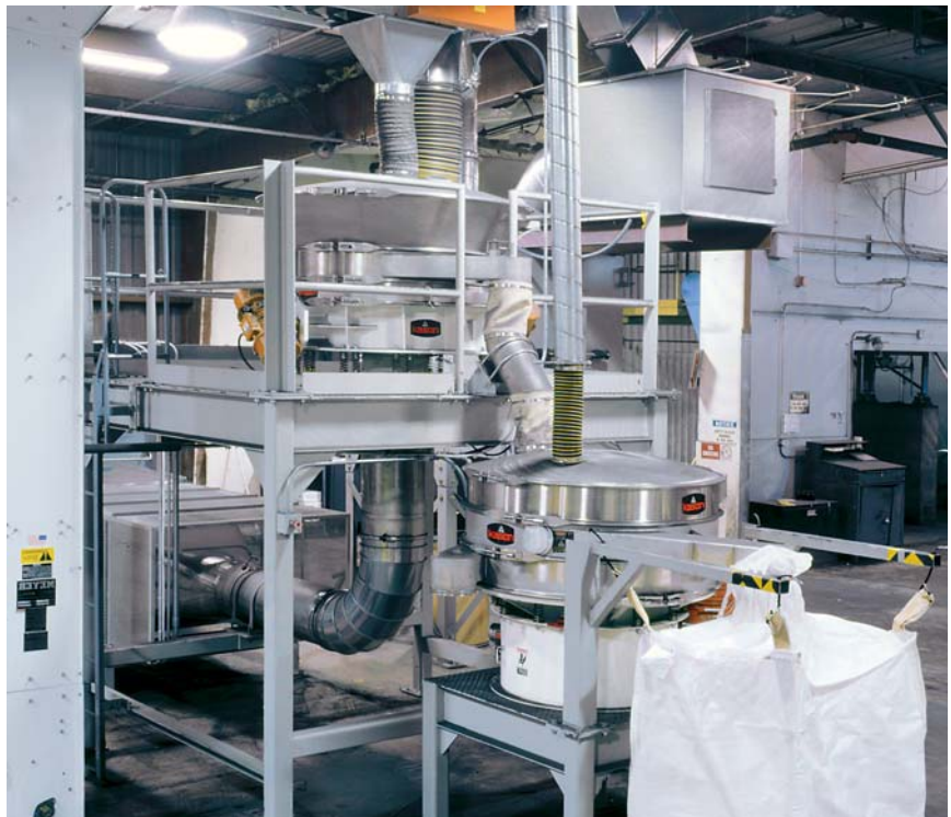
This skid-mounted, turnkey dryer/screener system configures a 48-inch (1225 mm) Fluid Bed Dryer and two-deck Circular Vibratory Screener in series to dry proprietary chemical powder while removing undersize and oversize particles at the rate of 2000 lbs/h (907 kg/h). The screener is equipped with a bulk bag hanger and extended discharge spout to align with the bag intake spout and magnetic ferrule to remove tramp metal from the finished product prior to packaging.
