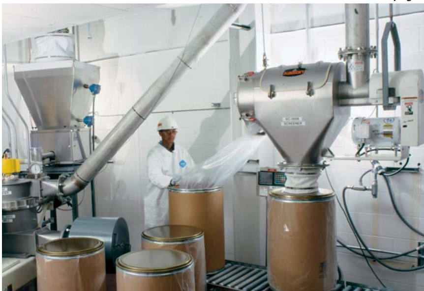
The Custom Services Group of Solvay Solexis cryogenically screens ground plastic resins at temperatures of -50° to -275°F (-46° to -170°C), placing extreme demands on its centrifugal screening equipment.
