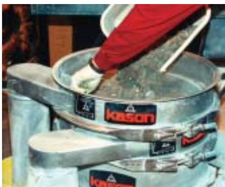
Dental laboratory scraps are unloaded into top 10-mesh screen of 24-in (610 mm) diameter Kason VIBROSCREEN® circular vibratory separator.
