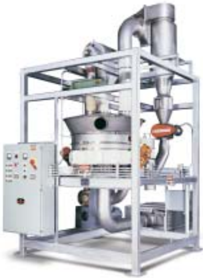
This 48-in (1220mm) diameter fluid bed dryer reduces moisture content of 50-mesh size ceramic particles from 7% to 2% at a continuous rate of 1000 lb/hour (454kg/hour). Temperature remains below 100°C (212°F). In addition to a heater, blower and cyclone separator, this system incorporates a CENTRI-SIFTER® centrifugal separator upstream of the fluid bed unit for continuous de-agglomerating of incoming material.
